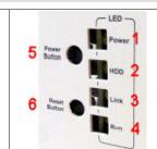
Power Button: Press and release to turn on the unit or shut down the OS and switch off the unit. Press and hold to switch off without OS shutdown. Reset Button: Triggers a hardware and PCI reset. The unit is restarted.
