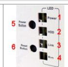
Power Button: Press and release to turn on the unit or shut down the OS and switch off the unit. Press and hold to switch off without OS shutdown. Reset Button: Triggers a hardware and PCI reset. The unit is restarted.
